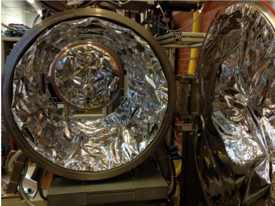
Figure 3.5 Multi-layer insulation inside the LISA chamber when first applied.
