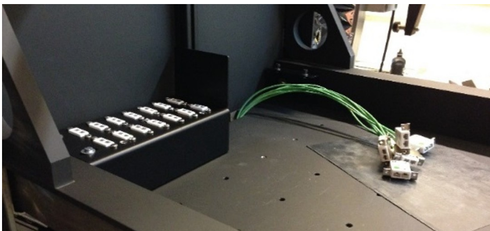
Figure 3.6 Thermocouple connection box used in earlier experiments with the cold plate and shroud.
